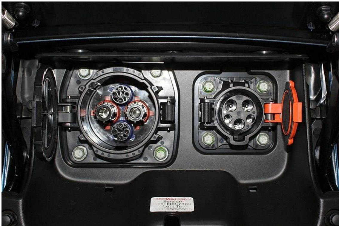
Figure 3. CHAdeMO and SAE J1772 (Type 1) Connectors in a Nissan Leaf
